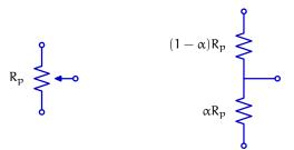
For each of the circuits on the following page, sketch a graph of the voltage drops across  $B_1$  and  $B_2$  versus  $\alpha$  (note that you do not have to solve for this relationship exactly).
