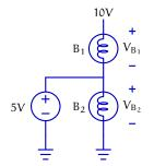
Now, we wish to use a  $10k\Omega$  potentiometer to provide the bulbs with a variable voltage, as we did in lab.
