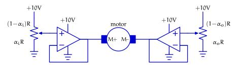
The dependence of the pot resistances on shaft angle is given in terms of  $\alpha$ , which varies from 0 (most clockwise position) to 1 (most counterclockwise position). The resistance of the lower part of the pot is  $\alpha R$  and that of the upper part is  $(1 - \alpha)R$ .
