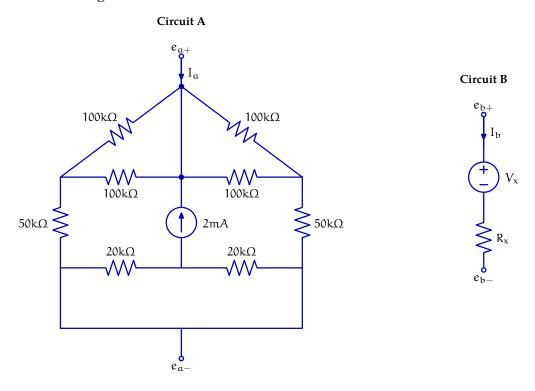
Let  $V_a=e_{a+}-e_{a-}$ , and let  $V_b=e_{b+}-e_{b-}$ . Determine values of  $V_x$  and  $R_x$  in circuit B such that the relationship between  $V_a$  and  $I_a$  is identical to the relationship between  $V_b$  and  $I_b$ .
