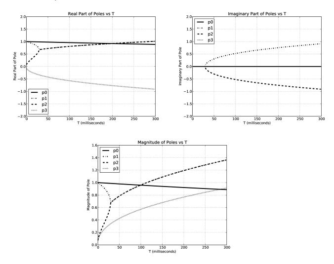
Note: The dash-dotted (p1) line and the long-dashed (p2) line overlap in part of the real and magnitude plots. The solid (p0) and the short-dashed (p3) lines overlap in the imaginary part plot.
