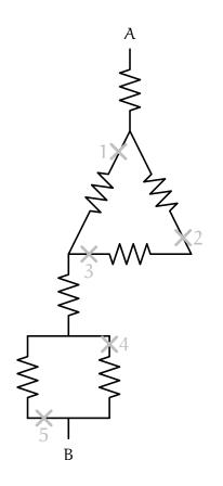
For each of the five locations, state whether cutting that wire would *increase* or *decrease* the resistance between the nodes labeled A and B, and by how much (in terms of  $R_1$  and/or constants). In each scenario, consider cutting the wire at that location *only* (in the absence of other cuts).
