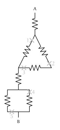
For each of the five locations, state whether cutting that wire would *increase* or *decrease* the resistance between the nodes labeled A and B, and by how much (in terms of  $R_1$  and/or constants). In each scenario, consider cutting the wire at that location *only* (in the absence of other cuts).
