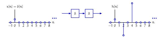
**1.** Calculate the first 6 samples of the response of the system  $\mathcal{H}$  to the following input signal:
