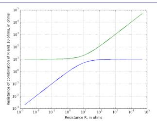
One curve represents the equivalent resistance of R in parallel with  $10\Omega$ , and the other represents the equivalent resistance of R in series with  $10\Omega$ . Which is which?
