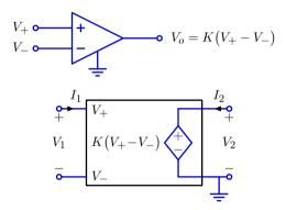
$I_1 = 0$  and  $V_2 = KV_1$ , where K is large (typically  $K > 10^5$ ). Not what is actually in an op-amp! This is a model.
