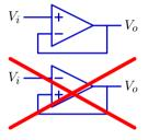
Takeaway: Feedback loop should go to the negative input of the op-amp.
