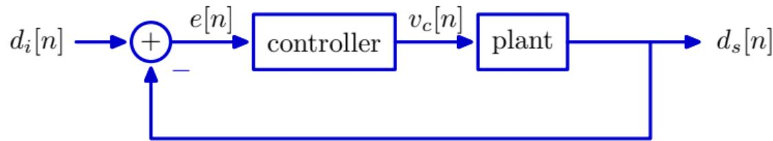
**Controller** (brain): sets commanded velocity  $\propto$  error:
